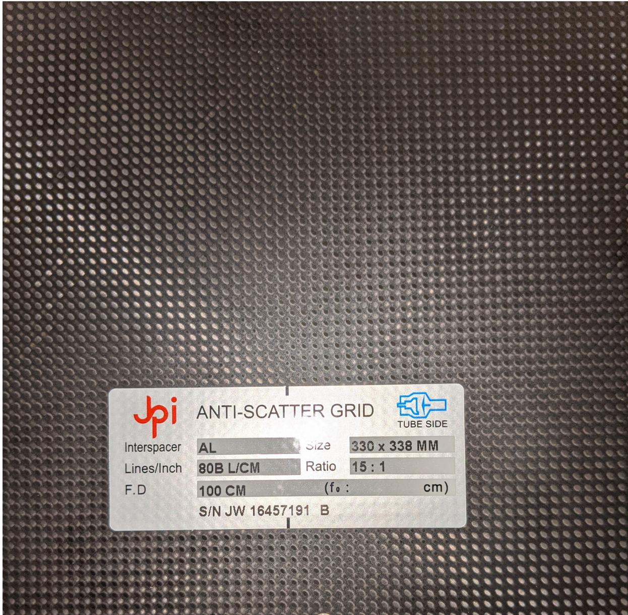
Figure 3.2: Picture of the grid equipped to the Alphenix detector.
