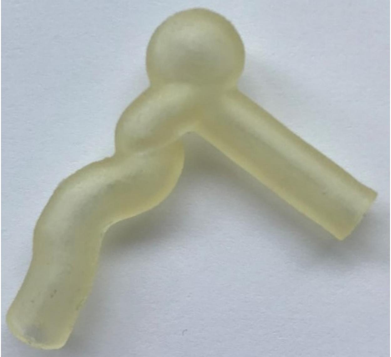
Figure 6.1: Picture of the 3D printed aneurysm phantom used to develop methods for flow measurements.
