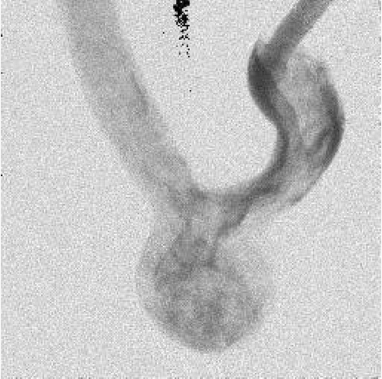
Video 5.5: 1000 fps HSA video showing blood flow detail in a saccular aneurysm phantom. Flow dynamic visualization improved by continuous x-ray exposure for 3 s. Video also available at: <https://youtu.be/1pIksOL11P8>.
